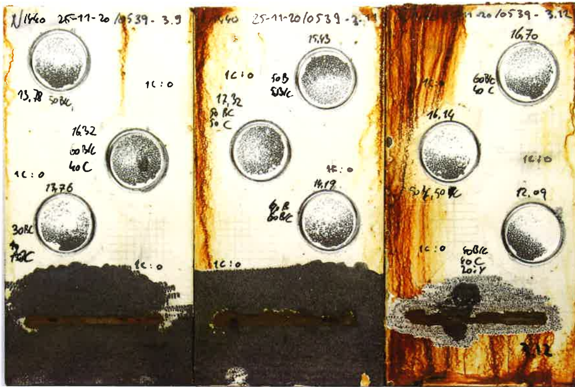
Photo 2a: Panels 3.9, 3.11 and 3.12 after 1440 hours Neutral Salt Spray test
