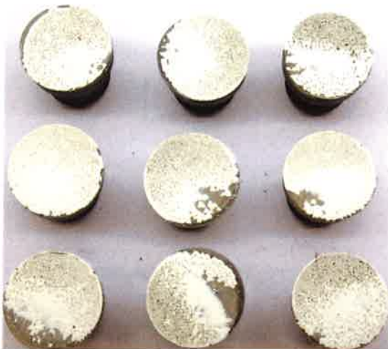
Photo 3b: Pull-off adhesion dollies Condensation test
