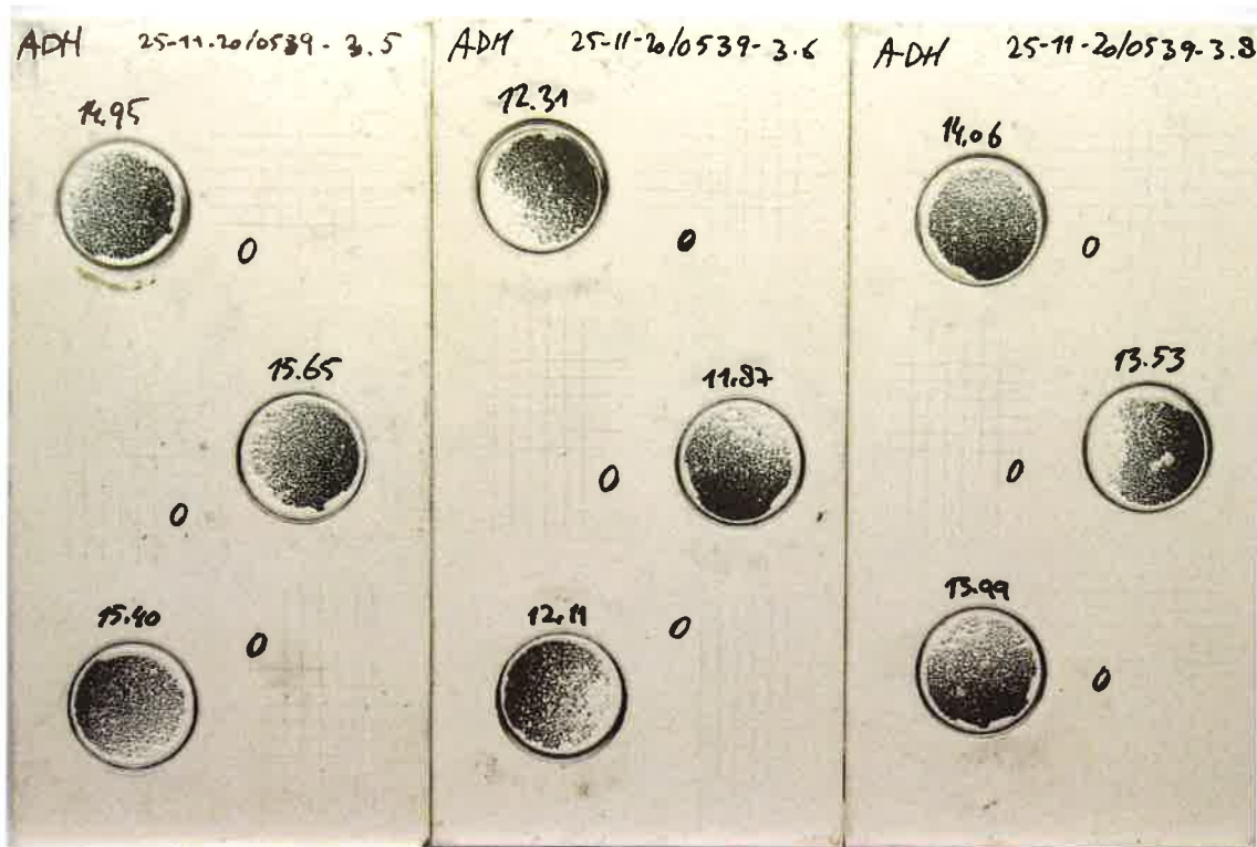
Photo 1a: Panels 3.5, 3.6 and 3.8 Reference adhesion
