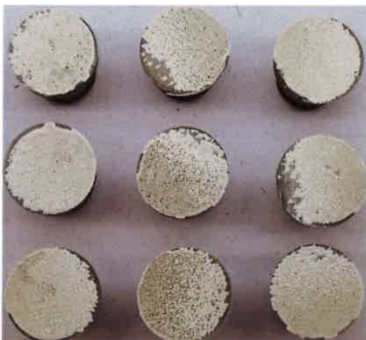
Photo 1b: Pull-off adhesion dollies Reference adhesion
