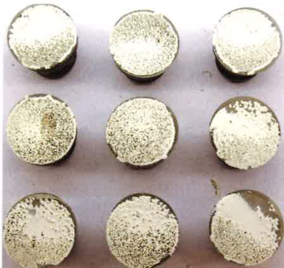
Photo 2b: Pull-off adhesion dollies Neutral Salt Spray test
